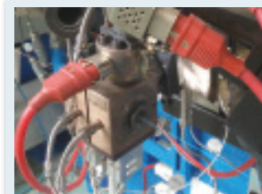
瑞士高精度双履共挤定心色条/色皮机头 Swiss high accuracy centered cross-head for color skin or stripping
