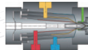
用作微米调节定心三层共挤机头时 Used for 3 layer SFS co-extrusion fix center cross-head with micro-adjustment
