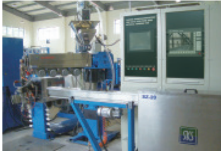
高质量螺杆及套筒, 保证出胶均衡, 线性良好。 Extruders are equipped with high quality screw and barrel to ensure homogeneous output with good linearity.
