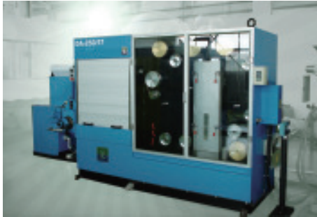
拉丝-退火-预热一体机, 退火及预热温度随速度自动跟踪, 采用德国整流装置。 Integrated wire drawing machine with continuous annealer and pre-heater. Automatic speed synchronization for annealing / pre-heating temperature.
