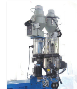
德国进口多种绝缘料自动配料系统 German made Multi-channel automatic dosing system for foaming insulating compounds
