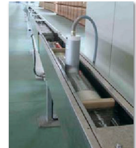
不锈钢双层水槽 Stainless steel made double layer thermal insulated warm water cooling trough
