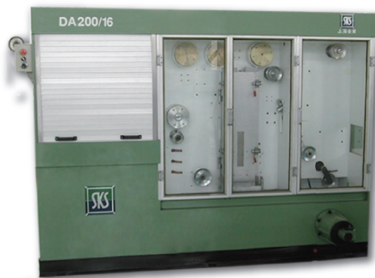
DA200 带连续退火铜线小拉机 COPPER WIRE DRAWING MACHINE WITH CONTINUOUS ANNEALER TYPE DA200 FOR FINE WIRE RANGE
